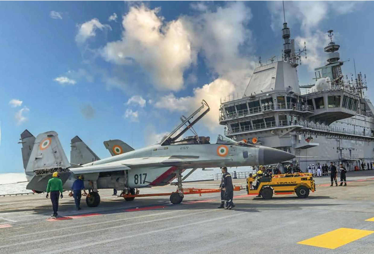
A MIG-29K aircraft of the Indian Navy is seen on the flight deck of the Indigenous Aircraft Carrier (IAC) Vikrant.
